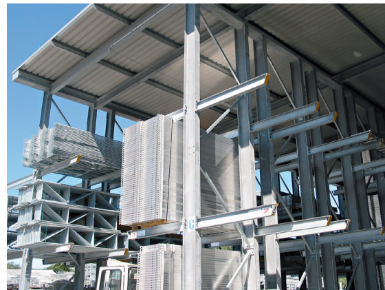
Hall with cantilever rack used on both sides
